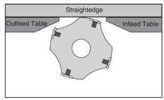
Figure 54. Infeed and outfeed tables adjusted even.
